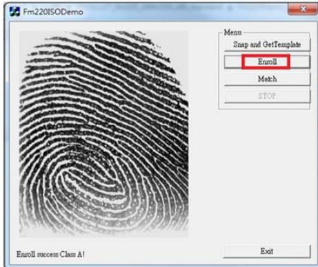
Step5. Press the Match button to begin matching the fingerprints of a user whose fingerprint data has been stored in the system. Press and remove the finger. Upon successful matching with the user's stored fingerprints, information is displayed with a score. When the captured fingerprint image size is 256x324, a score of 1500 and above ensures a security level with minimum FAR 1/100,000<sup>th</sup> and FRR 1/100.
